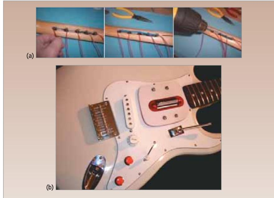
Figure 1. Taking a Guitar Hero video game controller apart and reassembling it inside a full-size electric guitar (a) Running wire to the buttons in the guitar neck. (b) The finished Guitar Hero controller.
