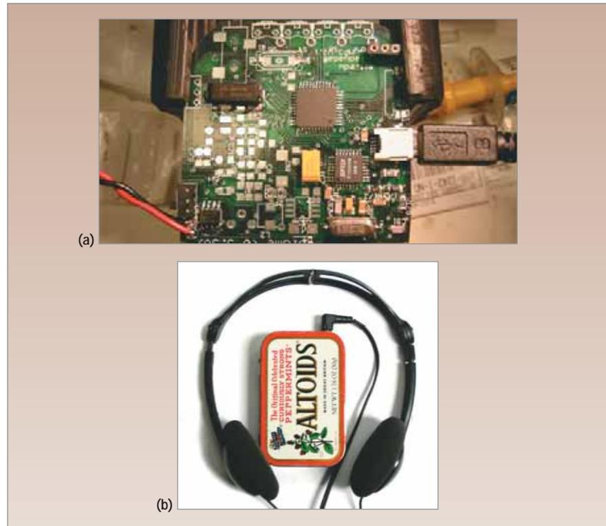
Figure 2. Assembling a MintyMP3 player. (a) Flashing the firmware. (b) The finished player.
